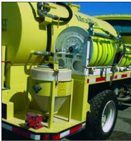
Chemical induction systems are now available on some sprayers, further reducing applicator exposure.
