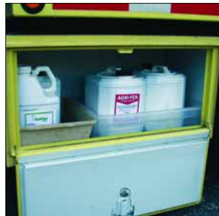
Secondary containment – On the truck, use plastic basins to line the base of your storage box. This will help keep containers upright and contain any leaks.
