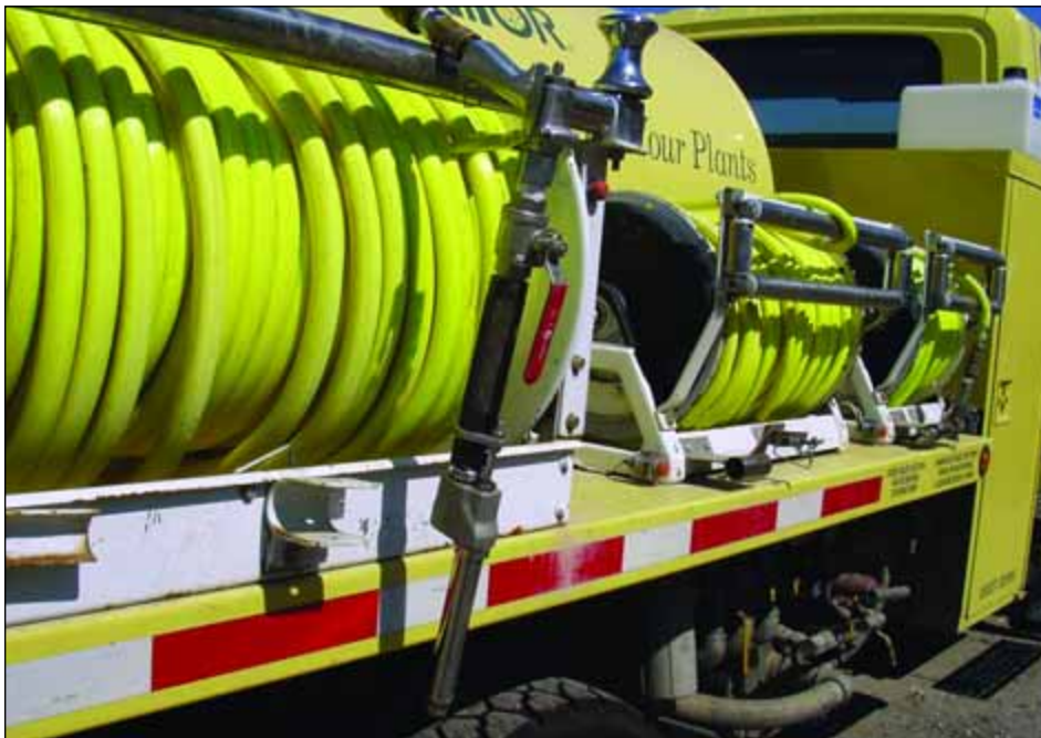
To facilitate staying close to the target, install a ball valve between the end of the hose and the gun or on the gun itself. This allows the applicator to cut down the volume, and effectively pressure, without going back to the truck.
